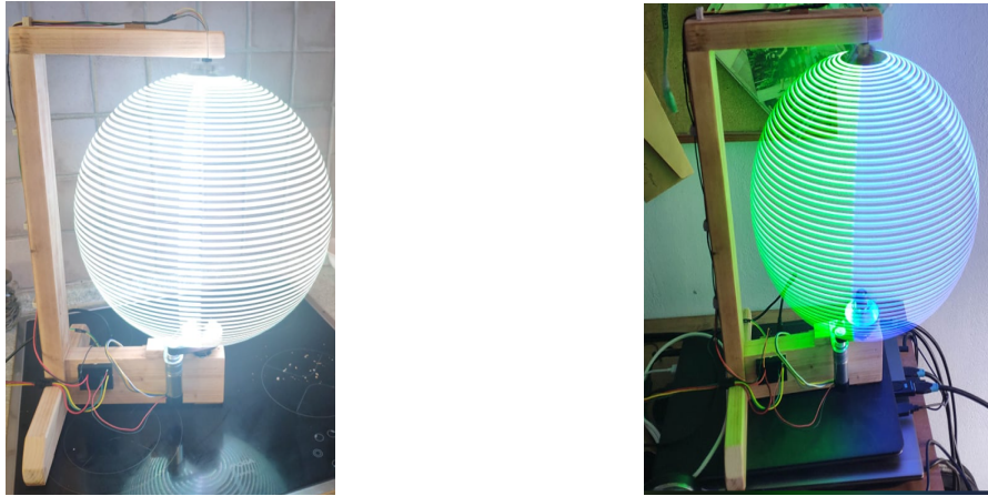
Figure 10. Right figure testing one color on display unit, left figure testing with 2 colors.
